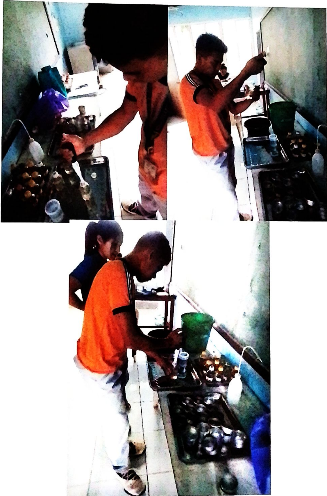
Figure 13. Collection of 20ml in every time of water samples collected and subjected for oven drying
