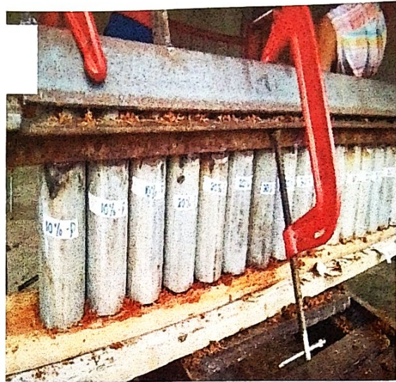
Compaction of briquettes using C-clamps
